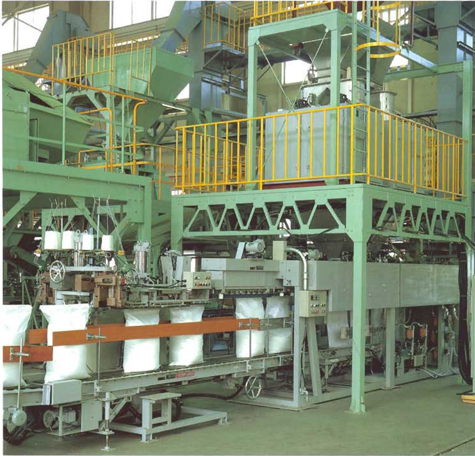
The photo shows Model 3CM-PD for bagging 40kg urea, using wovencloth bag. Two Duplex-scale installed overhead for a shop test at our factory before shipment.
