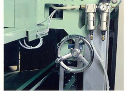
●Machine Height Adjuster Machine height is adjustable simply by turning the handle. The entire sealer rises or lowers, and can be locked at the desired height in a very short time.
