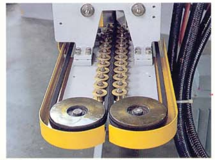
●Bag Support Belt Bags are transported without damage to the surface because they are supported between belts. The belts transport bags positively and smoothly.
